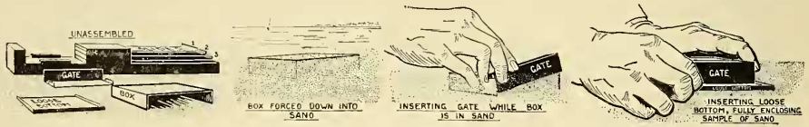
Fig. 1. See also Fig. 2. Apparatus for collecting layers of sand and mud on beaches, mud flats, and at the bottom of ponds, lakes and seas. The unassembled apparatus is shown at the left; its use in collecting is explained in the successive illustrations in Figs. 1 and 2, reading from left to right. All the operations except the last must be performed at the time of collecting. The last operation may take place in the laboratory. The rectangular collecting box, with two sides missing, is forced into the sand or mud. The two missing sides (gate and loose bottom) are then inserted, as shown above. To insert the loose bottom the adjacent sand is pawed away.
